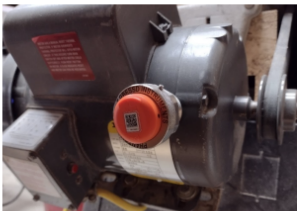
Figure 4. Phantom sensor mounted on the side of a motor housing (side-mount configuration).
