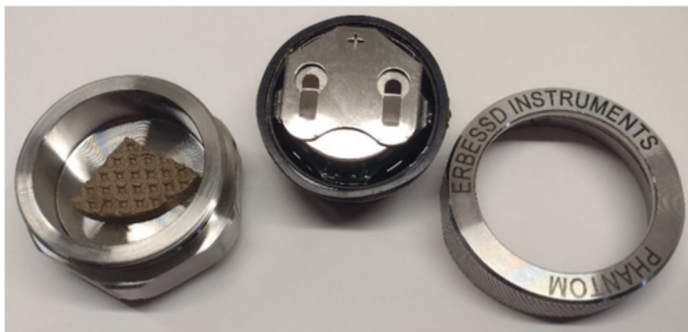
Figure 23. EPH-V11E sensor disassembled: base (left), sensor body with battery holder (center), and knurled ring with set screw (right).
