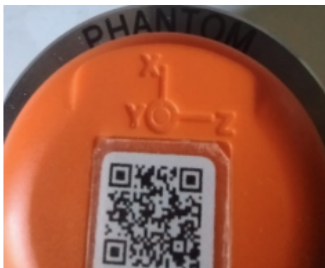
Figure 2. Axis orientation markings (X, Y, Z) embossed on top of Phantom sensor.
