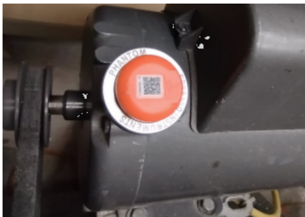
Figure 3. Phantom sensor mounted on top of a motor housing (top-mount configuration).
