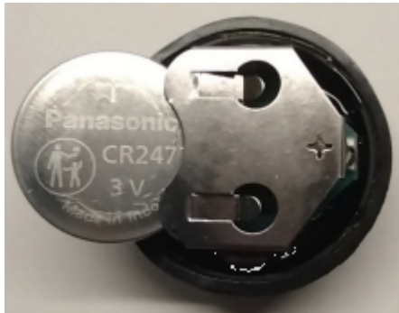
Figure 22. Panasonic CR2477 3V battery used in Phantom Expert Gen 3 sensors.
