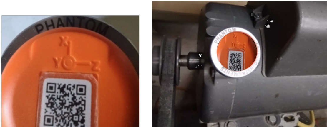
Figure 3. Axis orientation marker
