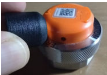
Figure 5. Magnetic “wake up” key
