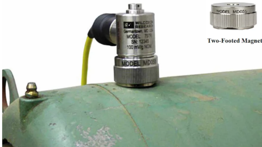
Figure 7. Example of a magnetically mounted accelerometer (image used courtesy of Wilcoxon)
