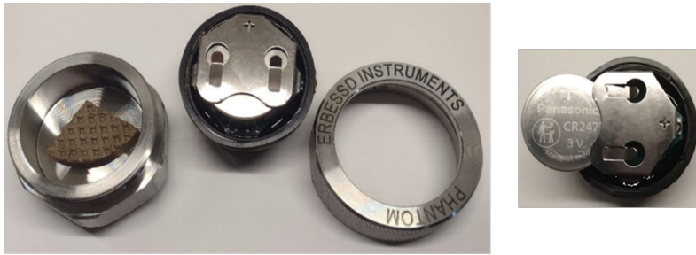
Figure 2. Phantom sensor parts with replaceable battery
