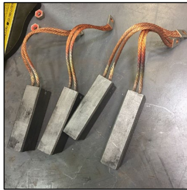
Figures 2 & 3: Discolored Leads – result of too much current on a given brush
