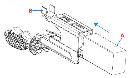
4. Insert the brush (A) the rest of the way into the holder until approximately 1/8 in (3.2 mm) extends out of the brush box.
