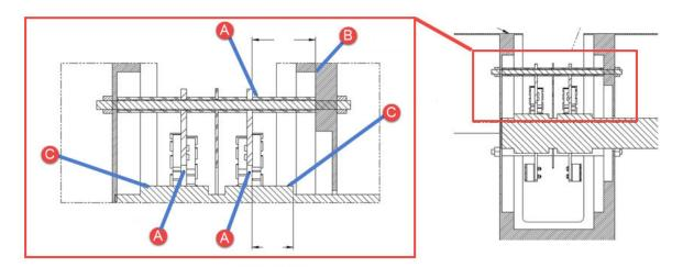
3. For confirmation, examine the brush position offset from the ring film to check for shaft growth. Note the difference from the running location.
