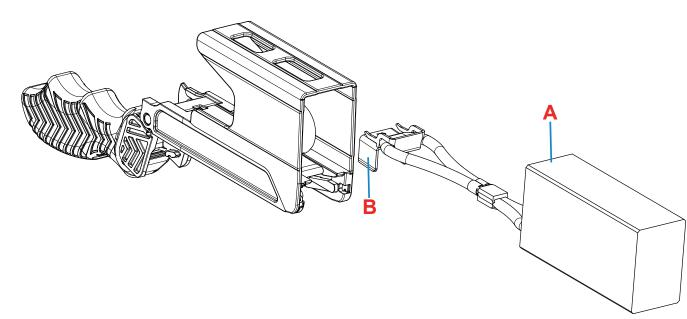
2. Insert the brush (A) into the holder (C) until the terminal ears (B) pass the brush spring.
