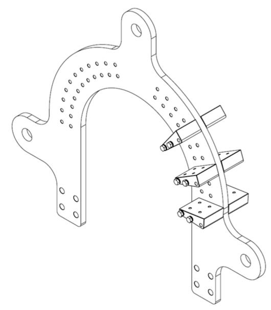
5. On the opposite side of the yoke, align and attach the adapters facing the opposite direction of the first three adapter pairs.
